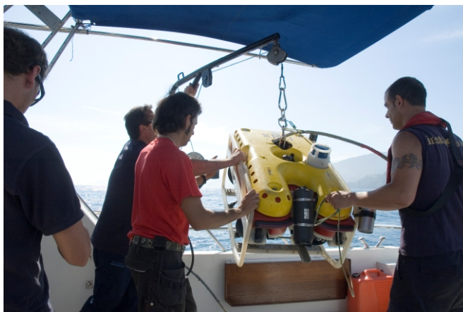
ROV operations for seabed and cable inspection at BIMEP (Credits AZTI).
