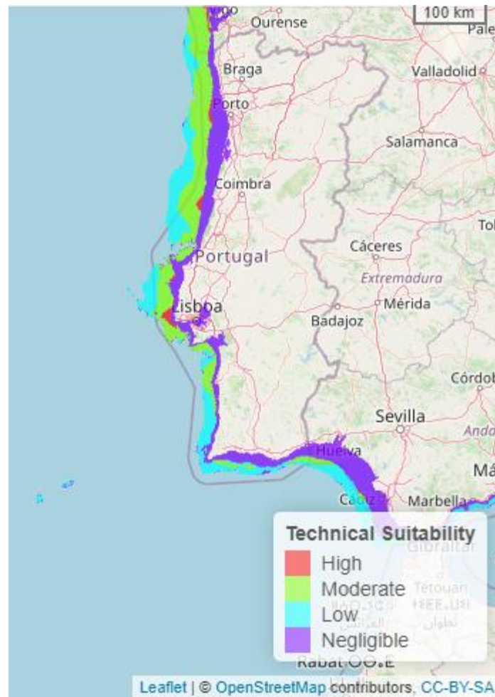
Figure 4. Technical suitability distribution for wave energy projects in the Portuguese mainland coast and southern Spanish Atlantic coast.
